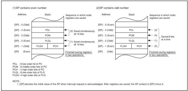
Figure 9.8 Operation of Saving Registers
